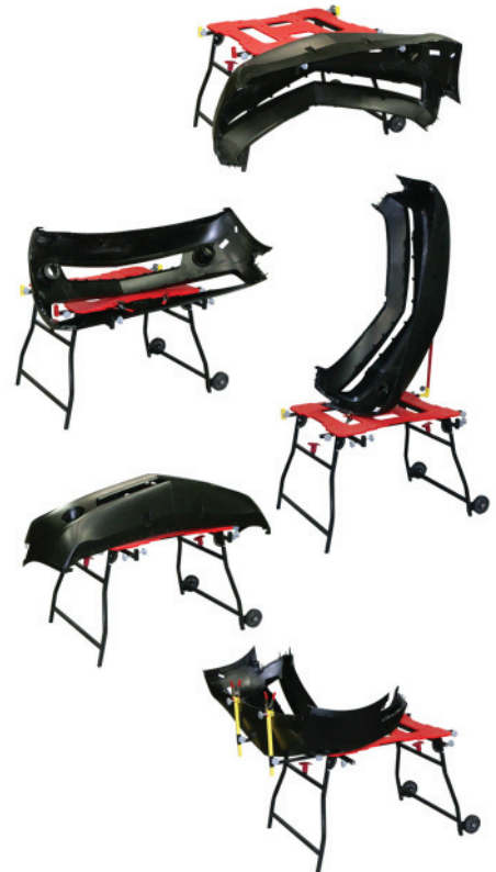
A sample of the many positions a bumper can be held in by the Bumper Mate.
