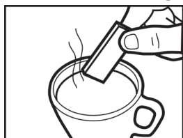
Place FlexMold bar in very hot water until it softens.
